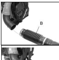
Assemble flexible pipe (B) to elbow
