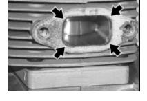
9. Stop engine, and re-tighten mounting bolts (or nuts) to specifications.
