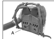
3. Install back cushion (A) to frame over intake cover.
