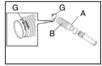
3. Assemble flexible pipe to elbow (D) on blower. Position clamp with cable guide loop (G) on outside of flexible pipe and tighten clamp.
