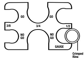
**Note:** Fitting and tube are not shown in illustrations for clarity. The Zurn PEX Crimp Gauge is to be used only on crimp rings that have been crimped onto tube and fittings.
