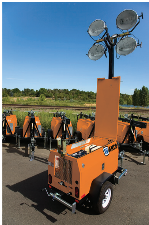
Hinged top panel opens fully. The light tower mast attaches to the panel for maintenance and raises the panel using the drawbar winch.
